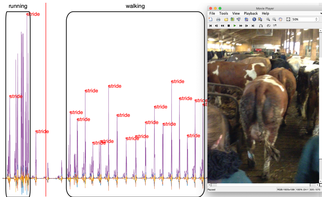
Fig. 3. The Annotation tool displays the squared magnitude of the accelerometer signal collected by a motion sensor attached to a cow. The individual strides of the cow have been annotated as event annotations (red) and the walking and running activities as range annotations (black rectangles).
