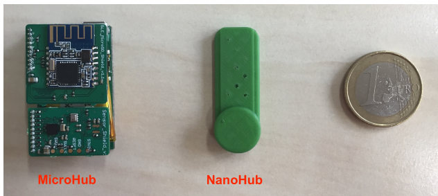
Figure 4. MicroHub (left) and prototype of the NanoHub (middle). Both devices contain a microcontroller, a 6-axis IMU, a BLE module and a battery. However, the MicroHub contains an additional SD card reader needed for development purposes.
