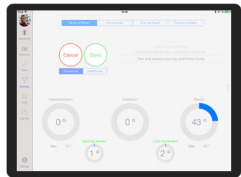
Figure 5: iOS App showing the angle of flexion of the leg.
