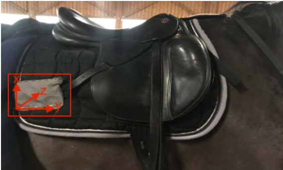
Figure 2. Placement of the smartphone on the horse’s body for measuring body movements during jump training.
