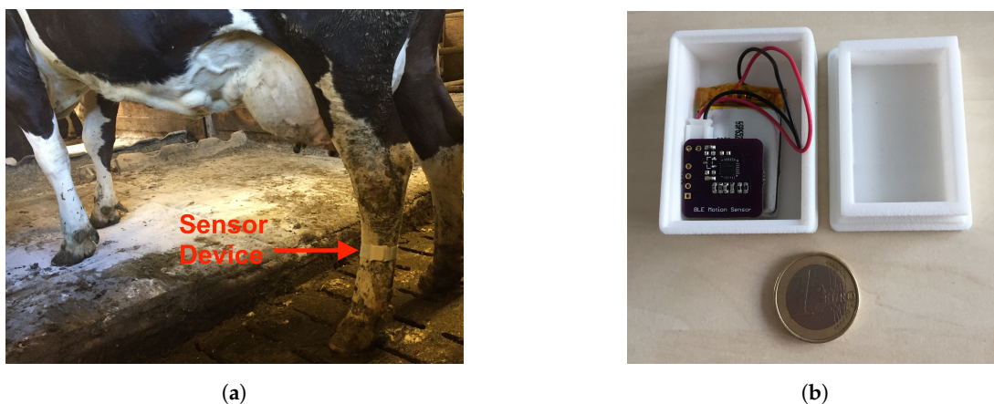
Figure 1. Motion sensor attached to a cow's hind left leg taken from [4,5] (a) and sensor box (b).
