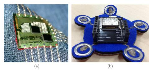
Figure 2.8: Electronic devices attached to fabric. (a) Flexible electronic module glued to the fabric and connected with embroidered conductive lines developed by the Fraunhofer's Institute for Reliability and Microintegration [71]. (b) Microcontroller connected with conductive thread to conductive snap buttons crimped. Developed in collaboration between the Technische Universität München and the Universität der Künste [45].
