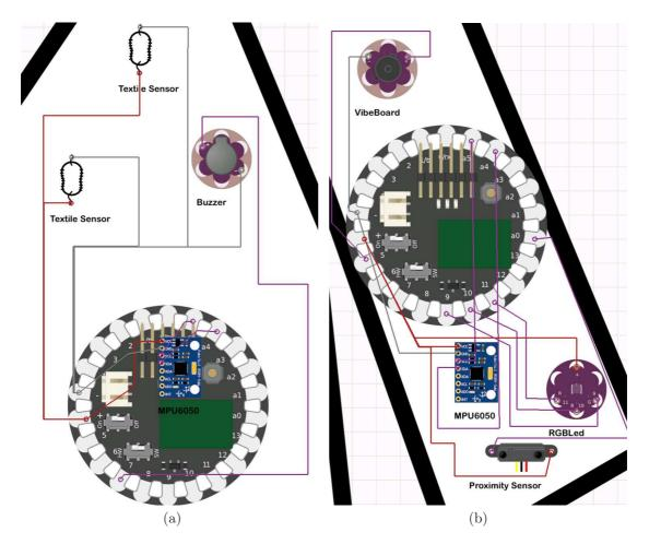
Figure 8.15: Circuit Design of the Custodian Jacket. a) Jacket's torso including Buzzer, Textile Sensor, Button, MPU 6050 and BLE-Lilypad. b) Jacket's Sleeve including MPU 6050, Proximity Sensor, Three-Color LED and BLE-Lilypad.
