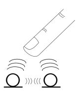
Optical fibers are flexible and transparent strands of plastic or glass. Due to the transparency of optical fibers, light can travel through them. Optical sensing works by measuring different properties of the light transmitted through optical fibers (e.g. intensity, wavelength), which can change due to external stimuli such as strain. The GTWM used optical sensing to detect wounds in military scenarios by detecting cuts in the optical fibers [95].
