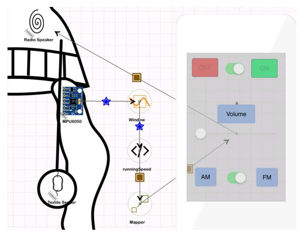
Figure 7.12: Usage of a *TextIT* plugin in *Interactex Designer* to control smartphone's volume based on estimated jogging speed.
