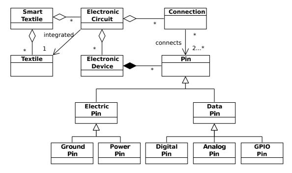
Figure 3.2: Model of a *Smart Textile*.
