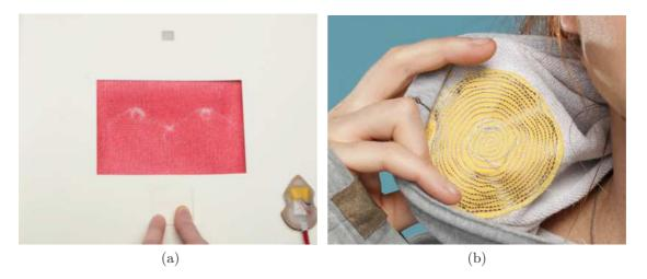
Figure 2.12: Textile output devices: a) Textile thermochromic display and b) textile speaker. Reprinted with permission of Katharina Bredies.
