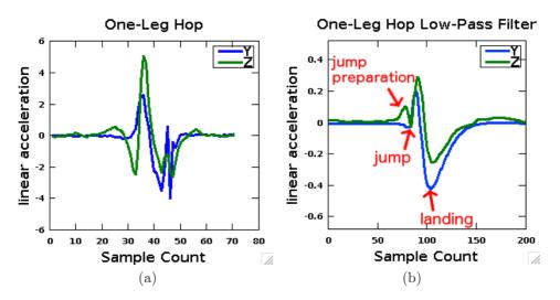
Figure 8.3: One-leg hop linear acceleration on y and z-axis raw (a) and filtered (b).
