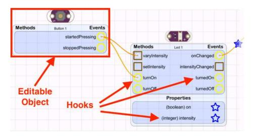
Figure 7.3: Invocations between Events of a Button and Methods of an LED.
