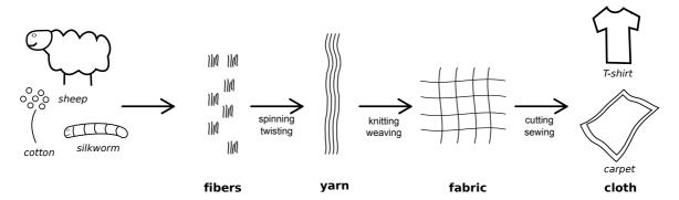
Figure 2.6: Textile fabrication process.
