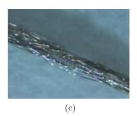
Figure 2.7: Different types of conductive yarns. (a) A copper foil wrapped around a non-conductive yarn. Reprinted with permission of Maggie Orth of *International Fashion Machines*. (b) A wire wrapped around non-conductive fiber strands [114]. Licensed under *Creative Commons BY 4.0*. (c) Multifilament yarn coated with a metallic layer [114]. Licensed under *Creative Commons BY 4.0*.
