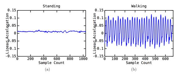
Figure 8.13: Linear acceleration along y-axis while user is standing (a) and walking (b).
