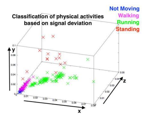
Figure 8.14: Classification of physical activities based on IMU data. Axes correspond to the deviation of the linear acceleration along the x, y and z-axes.
