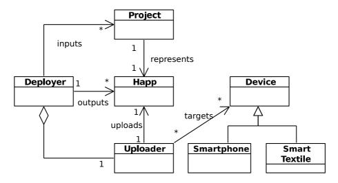
Figure 3.5: Model of the Deployer.
