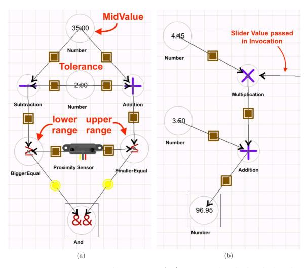
Figure 8.16: TangoHapps implementations of: a) Function that checks whether the proximity measured by a  $Proximity\ Sensor$  is in the range  $35\pm 2cm$ . b) Function that sets the color of the  $RGB\ LED$  to red.
