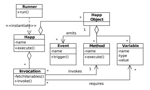
Figure 4.1: Main classes of the Running Engine.
