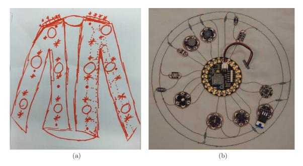
Figure 9.2: a) A paper prototype of a jacket developed during the Study 1. b) Textile testbed containing two accelerometers, a push button, switch, light sensor, buzzer, vibration motor and a three-color LED. Every electronic device is connected with conductive fabric to a custom-made Arduino Lilypad with an integrated BLE module (in the center).
