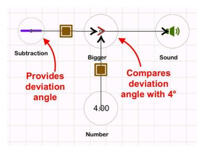
Figure 8.8: KneeHapp's functionality to produce auditive feedback when the user's knee deviates more than 4 degrees during a *One-Leg Squat*.
