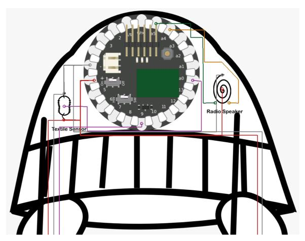
Figure 7.13: Circuit layout of WaveCap developed in Interactex Designer. Hardware Devices from left to right: a Textile Sensor, a BLE-Lilypad and a Textile Speaker (renamed to "Radio Speaker)".
