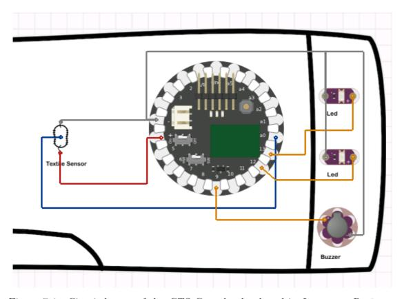
Figure 7.4: Circuit layout of the CTS-Gauntlet developed in Interactex Designer.
