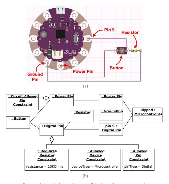
Figure 6.6: Layout (a) and object diagram (b) of an electric circuit that consists of a *Button* connected to an *Arduino Lilypad*.
