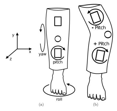
Figure 8.2: a) KneeHapp coordinate system. b) Illustration of the medial collapse during a squat. and how it affects the pitch.
