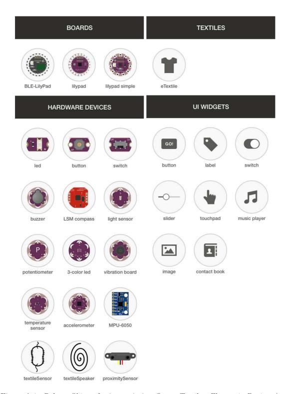
Figure A.1: Palette Objects for instantiating Smart Textiles, Electronic Devices (e.g. Hardware Devices and Microcontrollers) and UI Widgets available in Interactex Designer.
