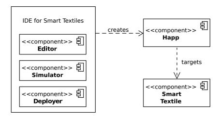
Figure 3.1: Main components of an IDE for smart textiles.
