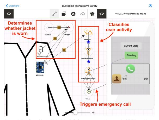
Figure 8.18: Custodian's *Technician's Safety* use case implemented with *TangoHapps*.
