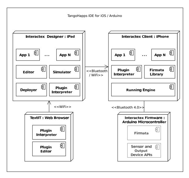
Figure 5.2: Deployment of software components in *THIDE*.
