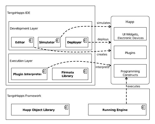
Figure 5.1: Software architecture of the THIDE based on the layered and repository architectural styles. The Happ subsystem is the repository. Software components in the  $TangoHapps\ IDE$  and  $TangoHapps\ Framework$  access the Happ. Accesses to the Happ are represented with dashed lines.
