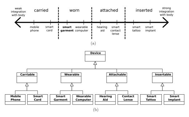
Figure 2.1: a) Smart garments compared to other devices according to their integration with the human body, based on previous work from Steve Mann [75]. b) Wearable devices represented as a taxonomy.
