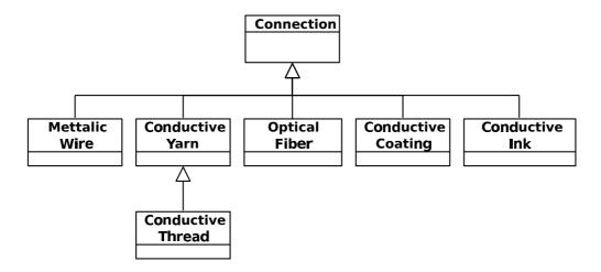
Figure 2.13: Taxonomy of connections used in smart textiles.
