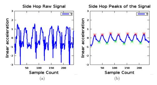
Figure 8.5: Linear acceleration of seven side hops. raw (a) and filtered (b).
