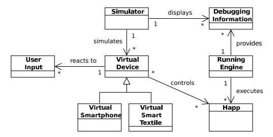
Figure 3.4: Model of the Simulator.
